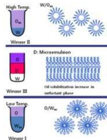
Figure 1. Mechanism of phase inversion zone depend on the temperature with (POE)12~20 fatty acid ethers of nonionic surfactants.
